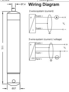
Note: Measurements are in mm. Cable not included (specify type and length) Note: Cable with integrated air tube for atomospheric pressure refill
