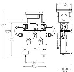
For differential pressure measurements at high line pressure (350 PSIG max), it is recommended that the pressure sensor be installed with a valve in each line, plus a shunt valve across the high and low (reference) pressure ports as shown.
