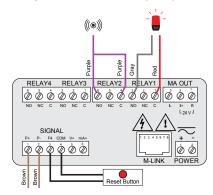
The PDA-LH5C shows one of five possible colors at a time. A typical application might use the green light to indicate everything is OK and the red light to indicate high and low alarms:
