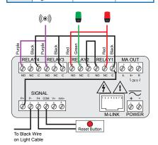
Indicate everything is OK with the green light, a High warning with the yellow light, and a High alarm with the red light. The Horn would also sound at both High warning and High alarms and can be manually reset at any time.
