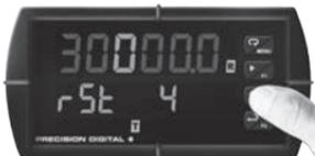
**Note:** Alarm #3 will set if the rate increases above 6,000 and will reset when the rate drops below 5,000. Use the 0-10 V simulator to demonstrate this. Alarm #4 will set when the total reaches 30,000 and will reset once the total is reset to zero. While the total is easily reset via the menu system, it can also be reset via a function key, or external digital input as shown below.
