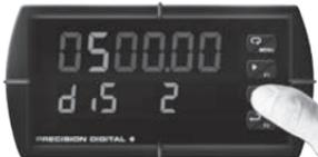
**Note:** To connect your transmitter to the PROVU demo, use the wiring diagrams provided on the back page of this manual. Connect the transmitter to the 24V supply using the P+ and P- terminals. Connect the 4-20 mA input signal from the transmitter to the mA+ and COM input terminals.
