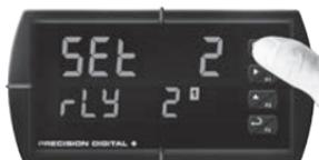
**Note:** The F3 button is programmed to function as an *Acknowledge Button* by default. Input 4 on the front panel of the demonstrator is programmed to function as F3 by default, so the digital input push-button labeled 'Input 4' may also be used to acknowledge the alarm.
