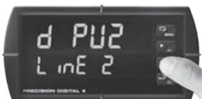
**Note:** PV2 will now be displayed on display line 2, where the units tag (*GR*) was displayed previously. Move the 0-10 V simulator up and down to demonstrate this capability.
