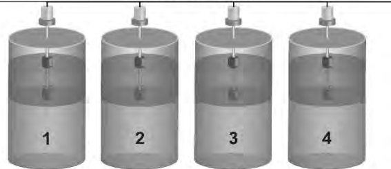
Tanks with Multivariable Level Transmitters
