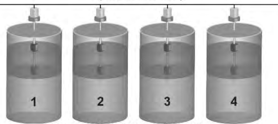
Tanks with Mutivariable Level Transmitters
