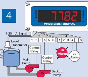
Relay #3 trips the High Level Alarm at 7500 gallons and resets at 6900 gallons.
