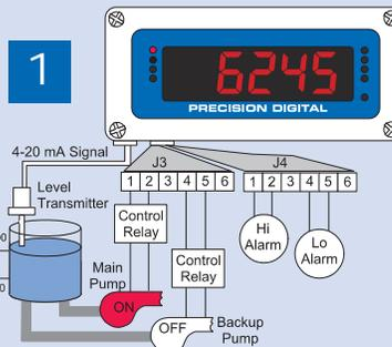
Relay #1 turns the main pump on at 6000 gallons and turns it off at 1000 gallons.
