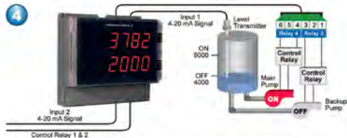
At 4000 gallons, relay 3 turns off and the system returns to normal pump alternation control.
