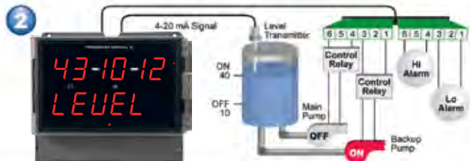
With the Pump Alternation feature activated, the next time the level reaches 40 feet, relay #3 transfers and starts the backup pump.
