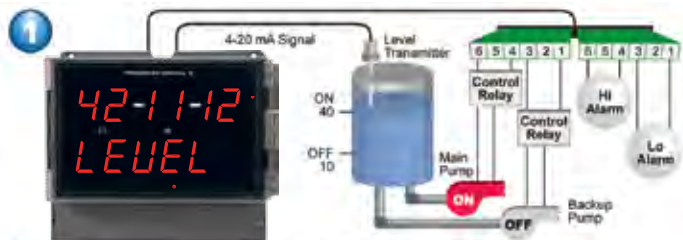
Relay #4 turns the main pump on at 40 feet and turns it off at 10 feet.
