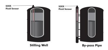
The S300-series can also be used with simple stilling wells and by-pass pipes to measure fluids.
