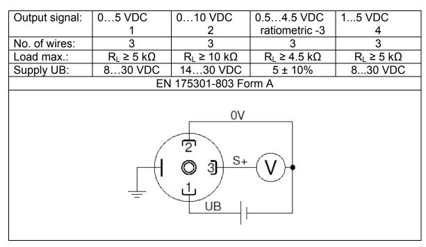
The transmitter metal case should always be connected to ground (GND) through the process connection thread in order to protect the sensor from disturbances due to electromagnetic fields or electrostatic charges.
