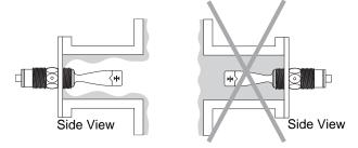
If installing the tuning fork within a pipe, make sure the forks allow the liquid to flow between them and not around them.
