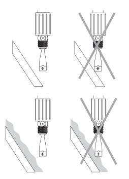
Higher viscosity liquids may build up inside of a flange and cause the NWP to fail wet.
