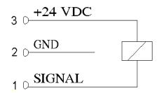
The reference point for the NPN-output is +24 VDC.
