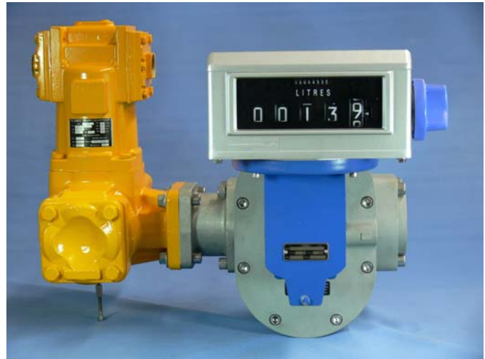
DOM series with Veeder-Root® 7887 reset register and optional air eliminator/strainer
