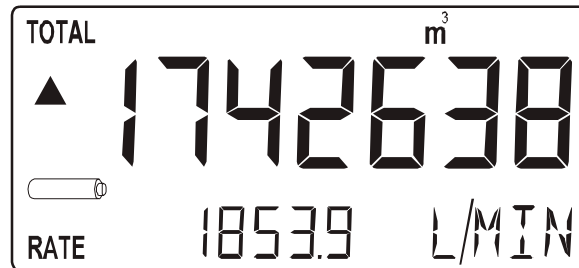
Fig. 4: Example of low-battery alarm
