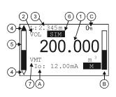
Measurement displaying with the NRM-300P display unit
