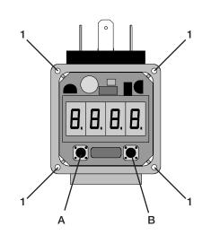
For adjustment, the 4 screws (1) of the display should be unscrewed and the cover removed.
