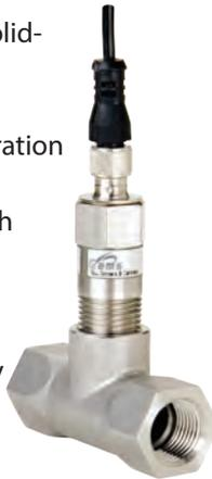
**TurboFlow®:** Ultra-compact TurboFlow® low flow rate sensors provide continual measurement ranging from 0.1 to 8 GPM (0.5 to 30 lpm). Their Hall-effect sensor delivers accuracy to  $\pm 3\%$  of reading and 0.5% repeatability. Lightweight, they mount in any position. Incorporate flow sensing into custom assemblies with the tiny TurboFlow® Insert.
