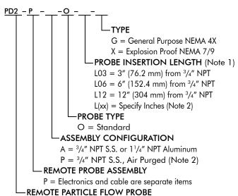
Note 1. For insertion length on  $1^{1}/_{4}^{\prime\prime}$  NPT mounting, add  $1^{1}/_{4}^{\prime\prime}$  (31.75 mm)
