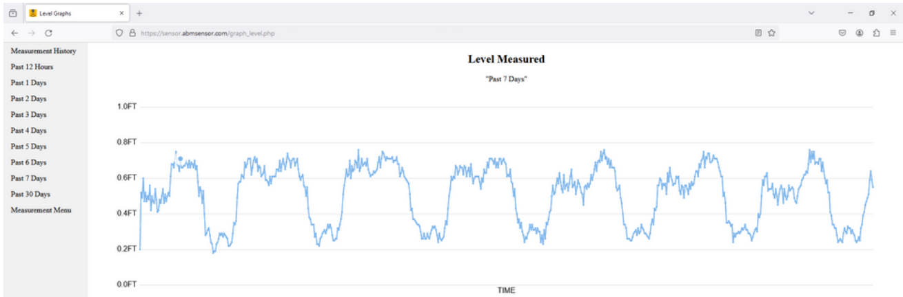
Figure 2: Historical level measurements from ABM’s radar sensor in a manhole tracking water levels in the sewer system.
