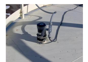
Application Problem: Radar unit has to have very narrow radiation beam to avoid false echoes from ship's body
