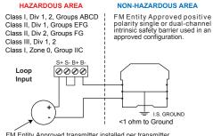
FM Entity Approved transmitter installed per transmitter manufacturer's Hazardous Location Installation Drawing PD688 & PD689 Entity Parameters:
