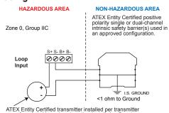
ATEX Entity Certified transmitter installed per transmitter manufacturer's Hazardous Location Installation Drawing.
