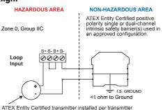
ATEX Entity Certified transmitter installed per transmitter manufacturer's Hazardous Location Installation Drawing. PD688 & PD689 Entity Parameters:
