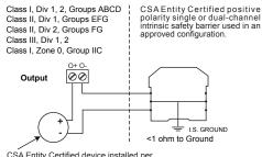
CSA Entity Certified device installed per manufacturer's Hazardous Location Installation Drawing. PD688 & PD689 Entity Parameters:
