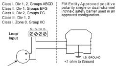
FM Entity Approved transmitter installed per transmitter manufacturer's Hazardous Location Installation Drawing PD688 & PD689 Entity Parameters:
