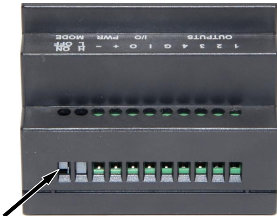
Figure 6. Normal Mode ON/OFF (Cascade Mode) Switch
