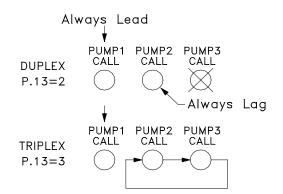
PUMP 1 ALWAYS LEAD Turns Off With Other Pumps On
