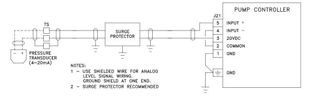
SUBMERSIBLE PRESSURE TRANSDUCER CONNECTION WITH INTRINSICALLY SAFE BARRIER
