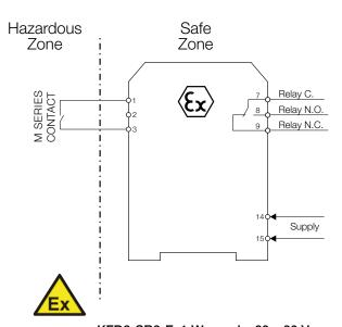
KFD2-SR2-Ex1.W supply:  $20...30 V_{DC}$  KFA6-SR2-Ex1.W supply:  $207...253 V_{AC}$
