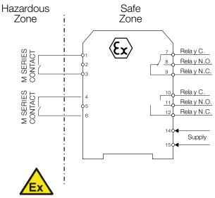
KFD2-SR2-Ex2.W supply:  $20...30 V_{DC}$  KFA6-SR2-Ex2.W supply:  $207...253 V_{AC}$
