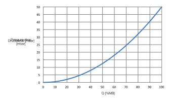
The diagram applies for gases with a density of air at NPT (0°C and 1013.25 mbar). The pressure loss is always proportional to the density of the gas. For example, the pressure loss doubles at 100% higher operating pressure.
