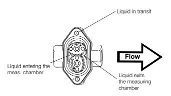
The positive displacement flow technology allows for precise flow measurement of most clean liquids regardless of the media conductivity. Other liquid properties also have a minimal effect on the performance of this type of meter. Flow profile conditioning is not required as with alternative flow technology options making oval gear installations simple to install in tight spaces and at an economical price.
