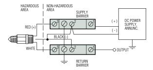
Supply and Return Zener Barriers used with GEMS ELS-1100 Series electro-optical level switch.
