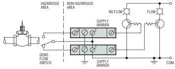
Used with GEMS flow switch located in a hazardous area for flow/ no flow indication.
