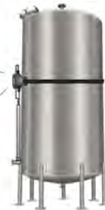
Non-invasive Ultrasonic Level Switch mounts on tank wall for point liquid level measurement. Easy installation and setup. Works on metal and plastic tanks with any liquid.
